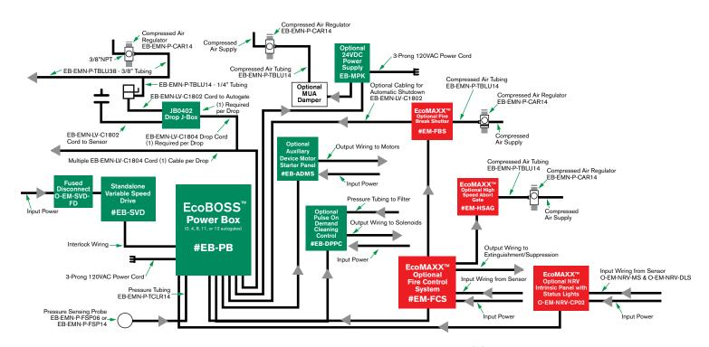
\*NOTE: Central Panel EB-IECP combines applicable Power Box system components in (1) Central Panel with Disconnect
