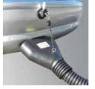
Adapters are critical to proper exhaust system function and for prolonging hose life. A hook and chain holds the adapter in place during use. At least 1/2" diameter difference between pipe and adapter is required for proper performance. Please refer to the information below for proper sizing.
