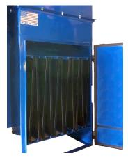
Carbon filter cell is used in cases where odors, gases, and vapors are associated with a process. Filter trays are removable and refillable. Activated carbon may be replaced with potassium permanganate. Available on models 1500 CFM and above.
